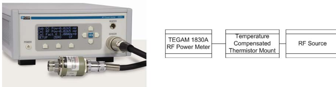
Figure 3 - TEGAM 1830A Method for Measuring Thermistor Mounts
